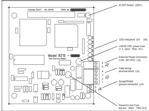
Figure 3-3: Model 8315 L&J Tankway Interface
